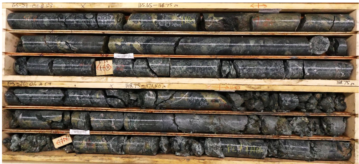
Figure 1: High grade Cu mineralization in GS26-06, showing most of a 7.5m interval of 3.72% Cu from 165m depth.
