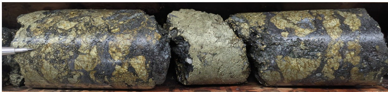
Figure 2: Massive chalcopryite and specular hematite at 45.2 m in GS26-02, within a 1m sample grading 9.87% Cu. Drill core is 6.3cm in diameter.
